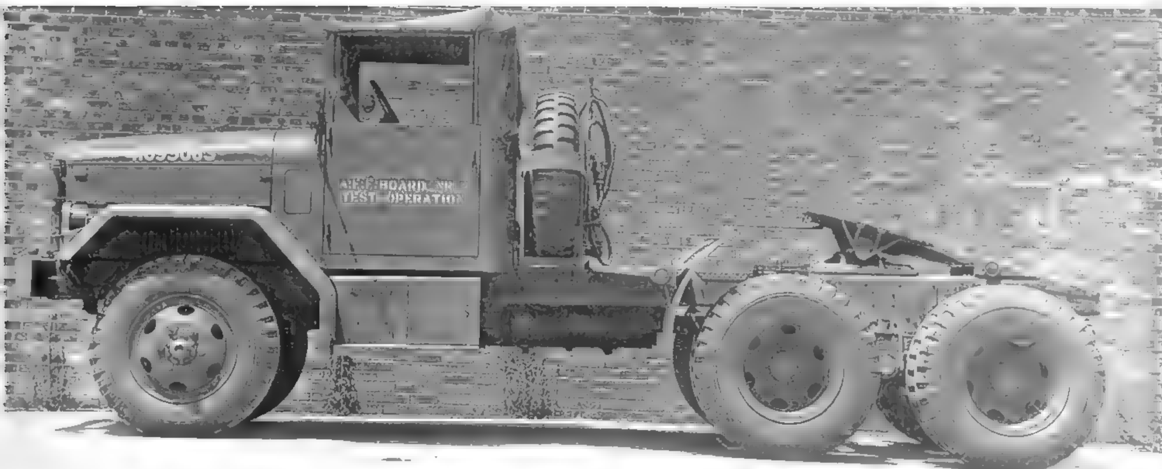
The M48 was the 154-in.-wheelbase tractor version of the G-742. A spare tire was carried behind the cab, and the trucks used the standard fuel tanks and toolboxes. (Photo courtesy of the Patton Museum)
